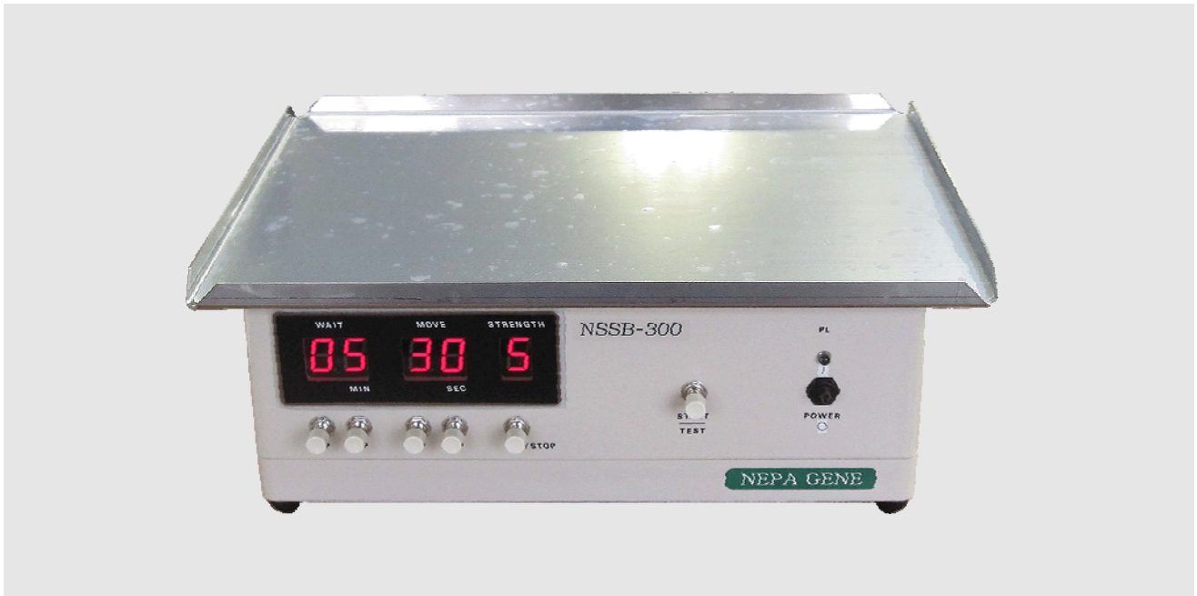
Figure 1. The NSSB-300 device (Nepa Gene, Ichikawa, Chiba, Japan) used for the mechanical agitation of the in vitro culture system. Petri dishes contain the fertilized oocytes, and embryos are placed in the machine's CO 2 incubator. Scale bar = 5 cm.
